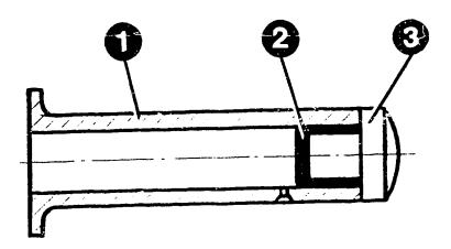
Press out plug (arrow) with mandrel. When pressing in appropriate plug, pay attention to tab washer or rubber sealing cap.
